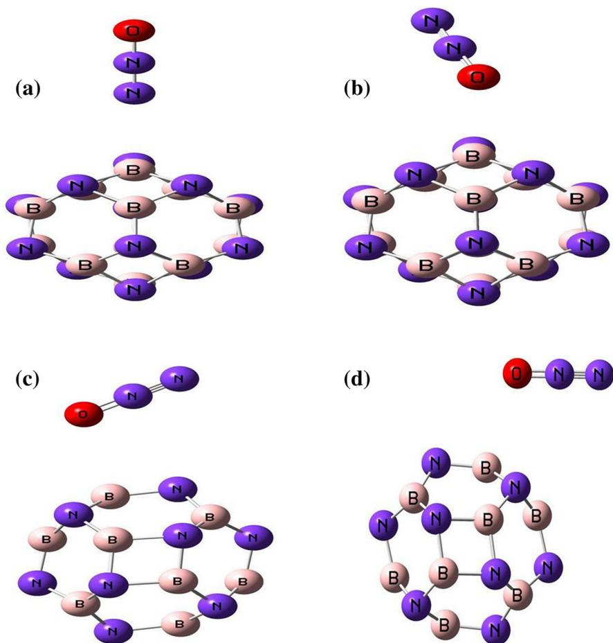
**Fig. 1** The optimized configurations of  $N_2O$  adsorption upon the  $B_{12}N_{12}$  by the nitrogen and oxygen attacking (a–d)
