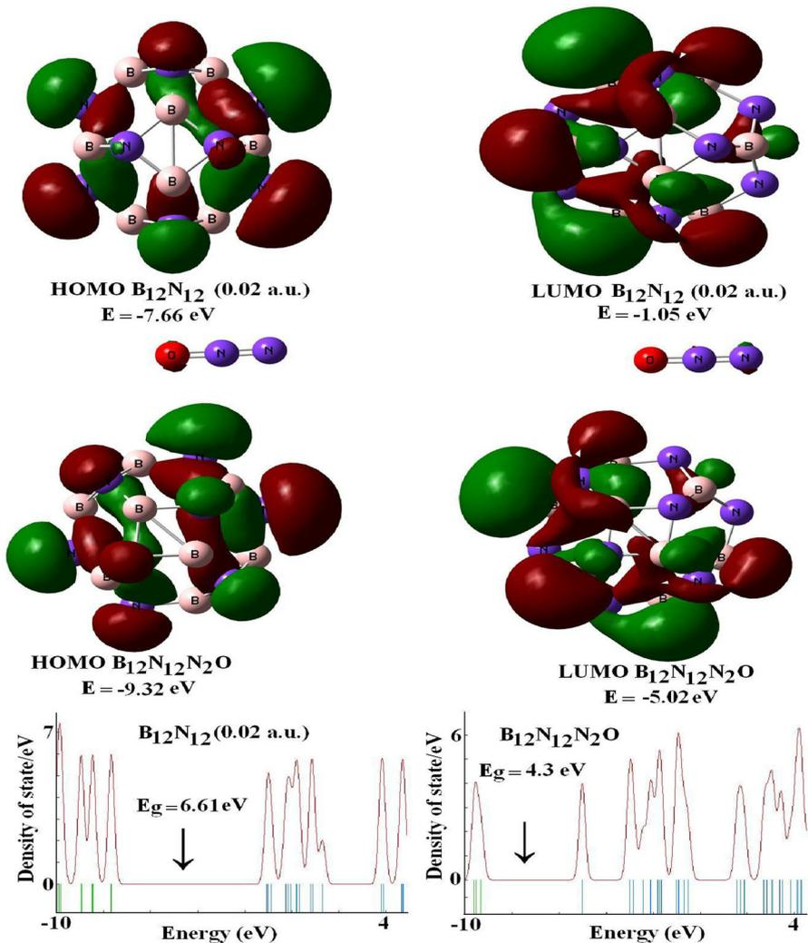
**Fig. 5** Profiles of the HOMO and LUMO orbitals of the pure B<sub>12</sub>N<sub>12</sub> and N<sub>2</sub>O/B<sub>12</sub>N<sub>12</sub> complex in the presence of an electric field
