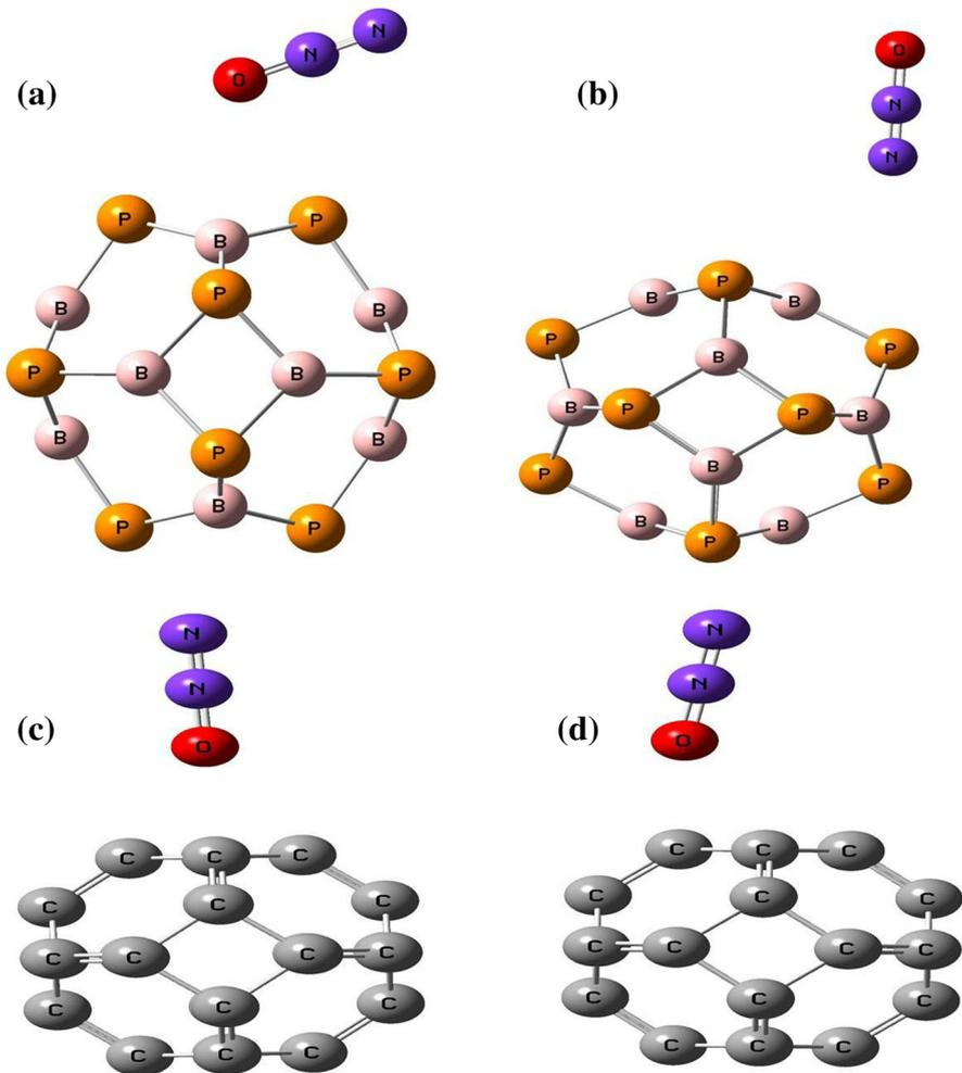
**Fig. 2** The optimized configurations of N<sub>2</sub>O adsorption upon the C<sub>24</sub> and B<sub>12</sub>P<sub>12</sub> by the nitrogen and oxygen attacking (a–d)
